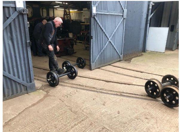
Wheel sets delivered to Alan Keef for brake work (Photos - Top Right Alan Titheridge, all others Tina Brown.
