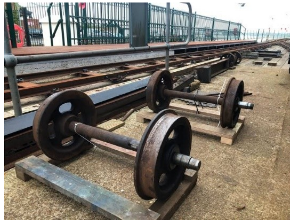
Wheels and axles from the carriage before being sent off for refurbishing.
